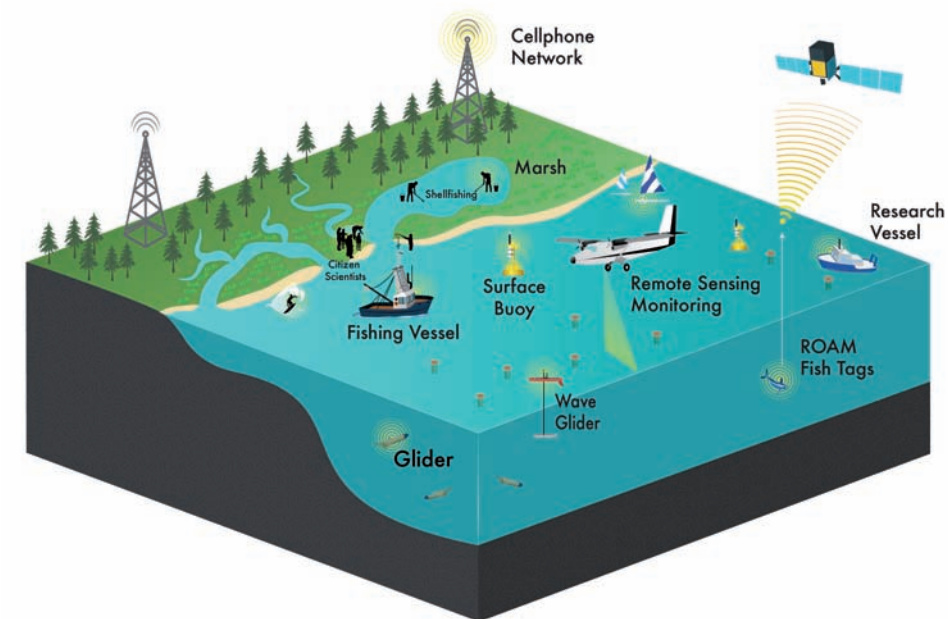
FIGURE 2. Schematic of the conceptual low-cost sensor network in the coastal ocean.
