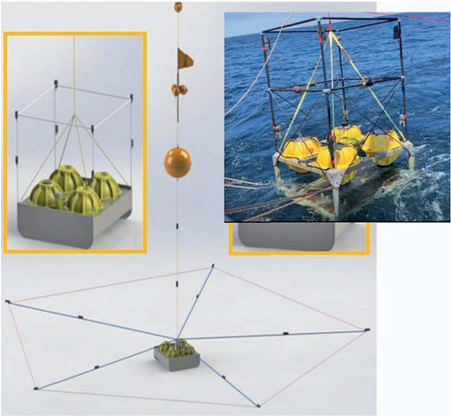
Example of a reconfigurable hydrophone mooring for ambient sound measurements.
