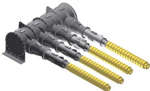
*GreenLink Hubs are heavy-duty, dry-mate modular 'subsea sockets' made up to house multiple cables. Each module is mechanically linked to other modules and extra sections can be added at initial launch or at a later stage, making the GreenLink Hub a flexible option over time.*
